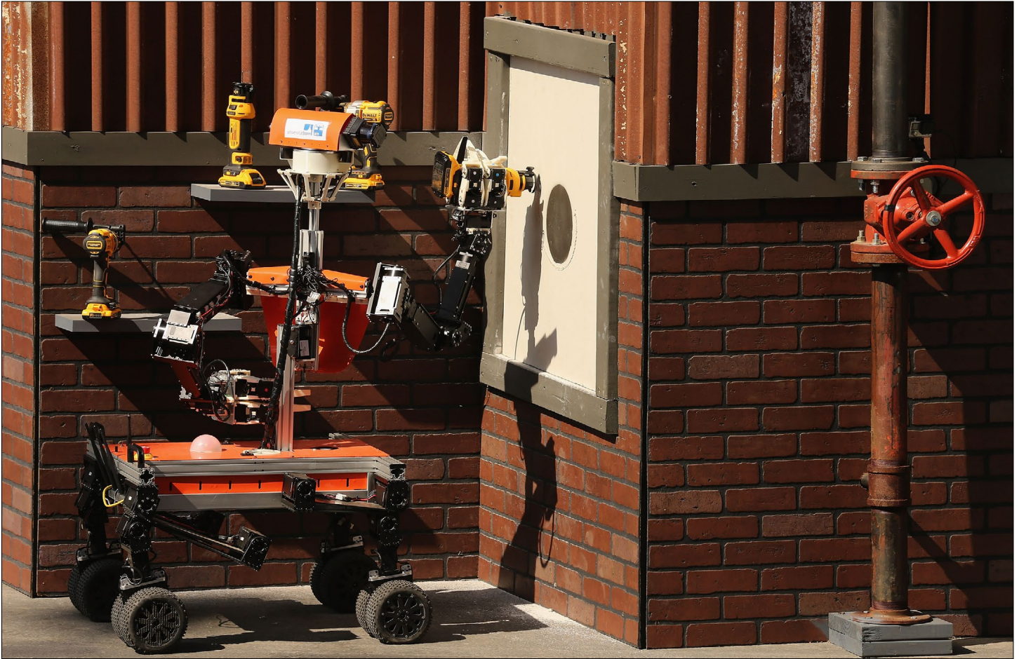
The Team NimbleRo Rescue semi-autonomous robot uses a power tool to cut through drywall during the Defense Advanced Research Projects Agency (DARPA) Robotics Challenge at the Fairplex June 5, 2015 in Pomona, California. (Chip Somodevilla / Getty Images)
